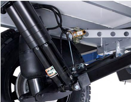
**Airbag suspension and disc brakes**
