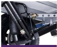
Airbag suspension and disc brakes
